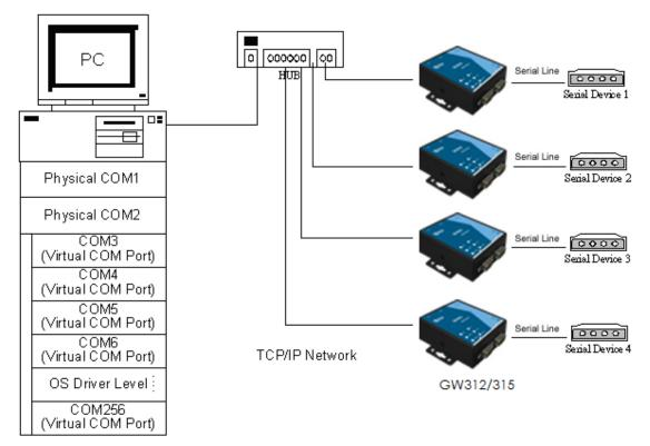
Fig. 35. Virtual Com connection diagram
